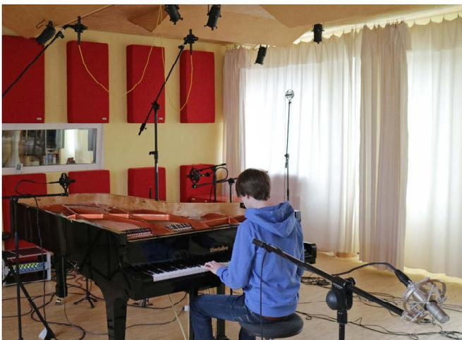
**Figure 4:** The 3D microphone setup for the grand piano in the studio. In the foreground the back left microphone, at the curtain the right side microphone.
