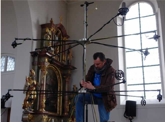
**Figure 3:** The first test setup with 13 cardioid microphones.
